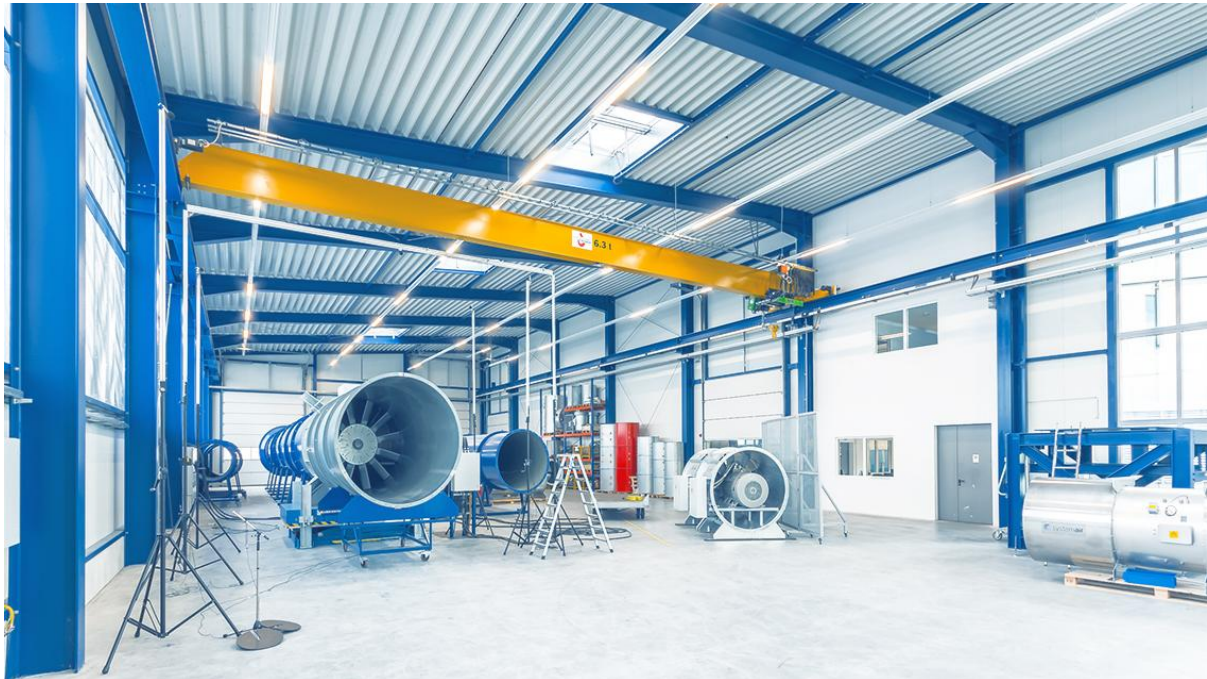
Figure 4. Duct test rig ISO 5801 ©Systemair
